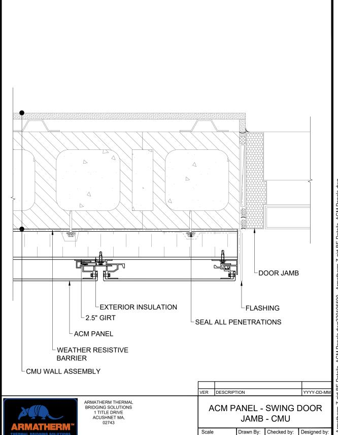
220195500 - Armatherm Z-girt BE Details\_ACM Panels.dwg220195500 - Armatherm Z-girt BE Details\_ACM Panels.dwg
